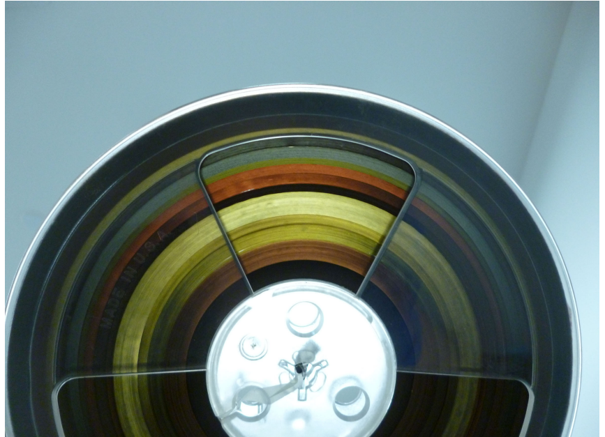
Image 1 Acetate tape spliced to polyester tape
